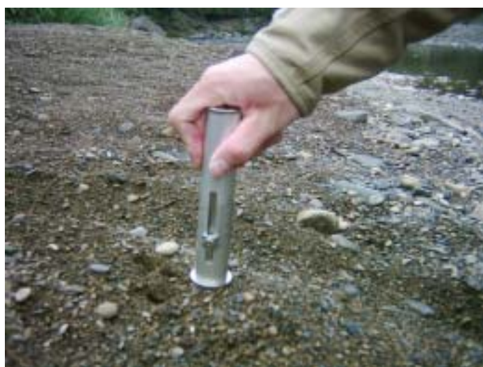
圖 4.2.8 山中式土壤硬度計 (Yamanaka's soil hardness tester , FUJIWARA SEISAKUSHO, LTD)
